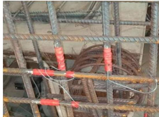
(a) Bottom steel reinforcement and electric strain gauges (ESG).
